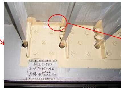
鋼床版部の疲労き裂
