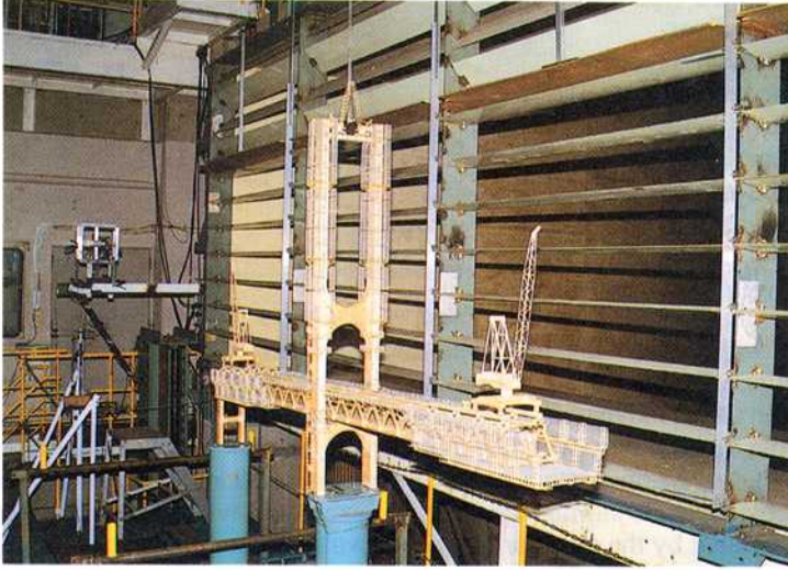
Figure 23. Wind Tunnel Test on Tower During Erection Stage
